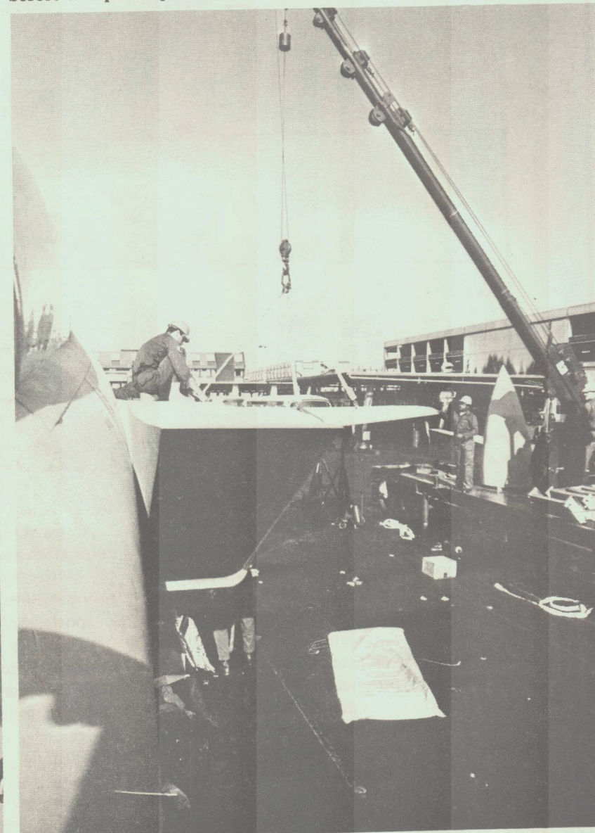
IN PLACE - A crane is used to secure the wing to the F-15. The procedure is much the same for securing the tail section. (U.S. Air Force Photo)
